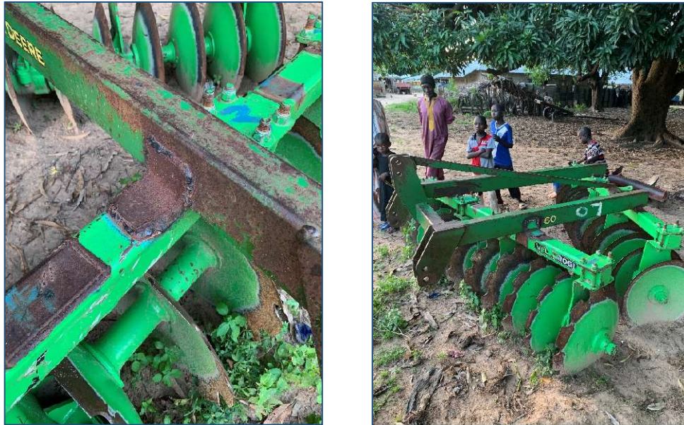
Figure 4. Community disc harrow showing replacement of frame
